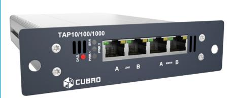
The Cubro 10/100/1000 Copper TAP allows the uninterrupted passage of full duplex data over standard Category 5/6 copper network cable. Featuring auto negotiating between 10Mbps, 100Mbps and 1000Mbps, this TAP duplicates the network signals, including any existing physical errors to the transmit-only monitoring ports.
